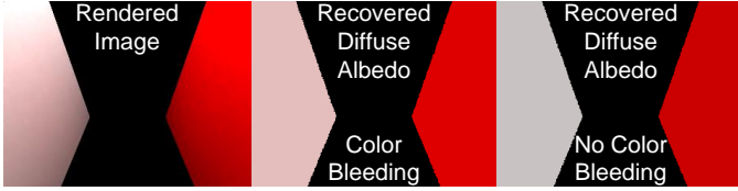
Fig. 15. Effectiveness of sufficient sampling constraint. There is a light source on the top, a white diffuse plane on the left, and a red diffuse plane on the right (left image). Color bleeding occurs without sufficient sampling constraint (middle image). The diffuse albedo is recovered correctly only with sufficient sampling constraint (right image)
